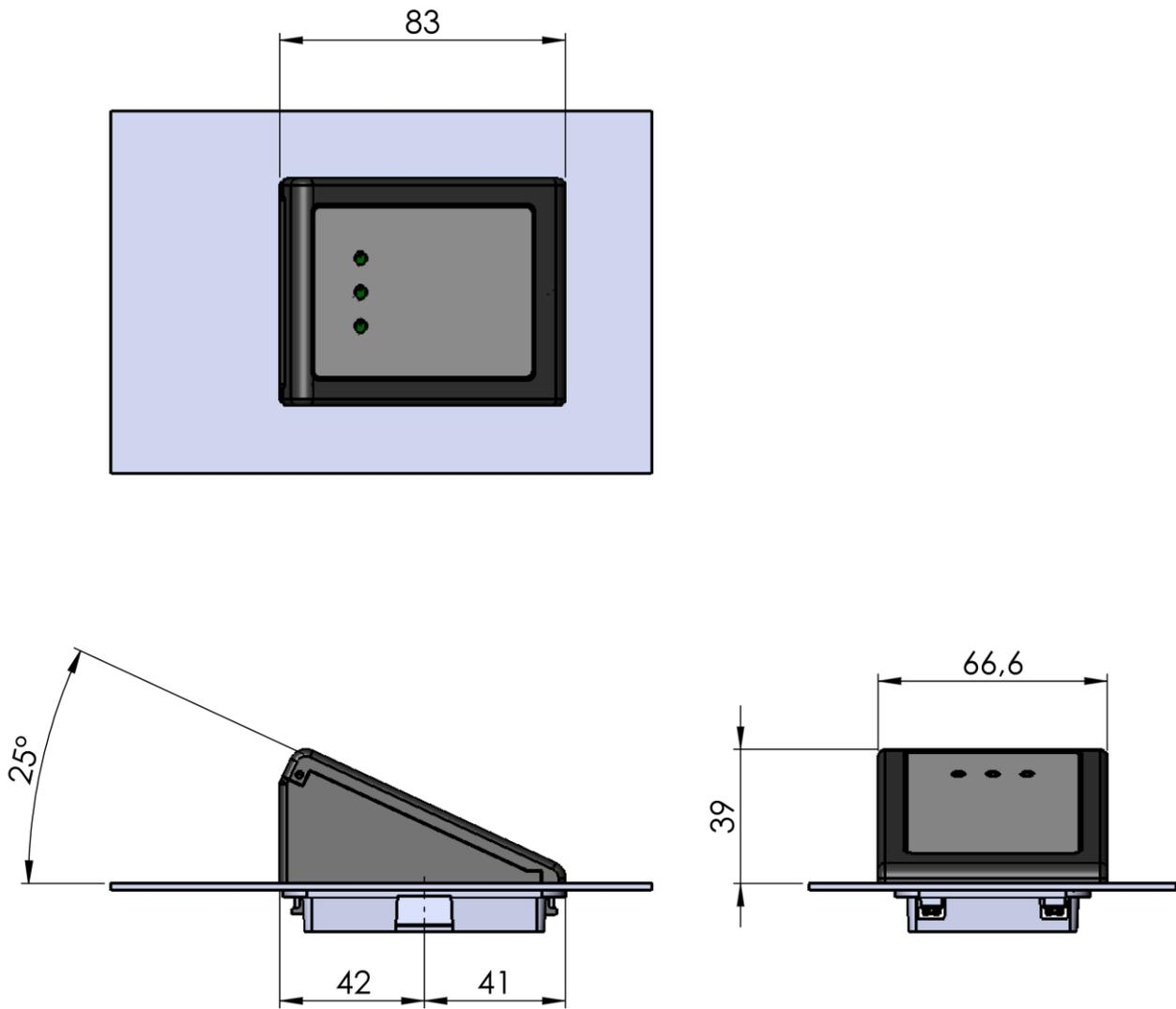
\*All drawing measurements in mm
