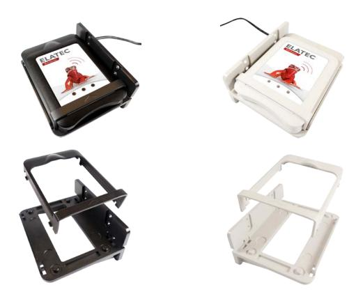
The TWN4 SmartCard Holder is a mounting kit to attach Elatec's TWN4 MultiTech SmartCard readers on a flat surface with screws (not included in the kit) or with a strong double sided adhesive pad (included in the kit). It is available in white and black color and consists of two parts which can be assembled for left or for right side mounting.
